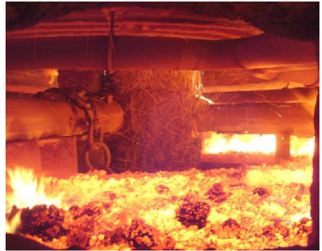
MHF WITH CIRCLE SLOT JETS
