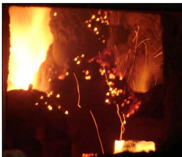
Figure 5. Comparison of Poultry litter Burn in MHF furnace without, and with, CSJs
